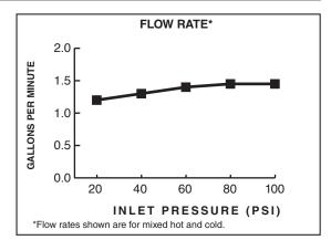
1.5 gpm/5.7 L/min. FLOW RATE
